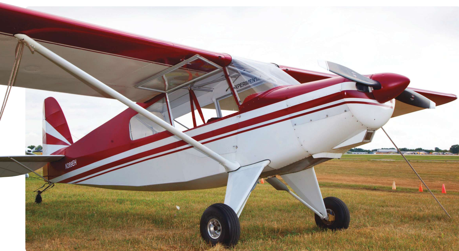
Wearing a signature Bob Barrows' maroon-and-cream paint job, the Bearhawk LSA clearly shows its family resemblance to Barrow's earlier four-place Bearhawk and two-place Patrol. The Bearhawk LSA originally flew with a Continental A-65 and showed outstanding climb and cruise.
