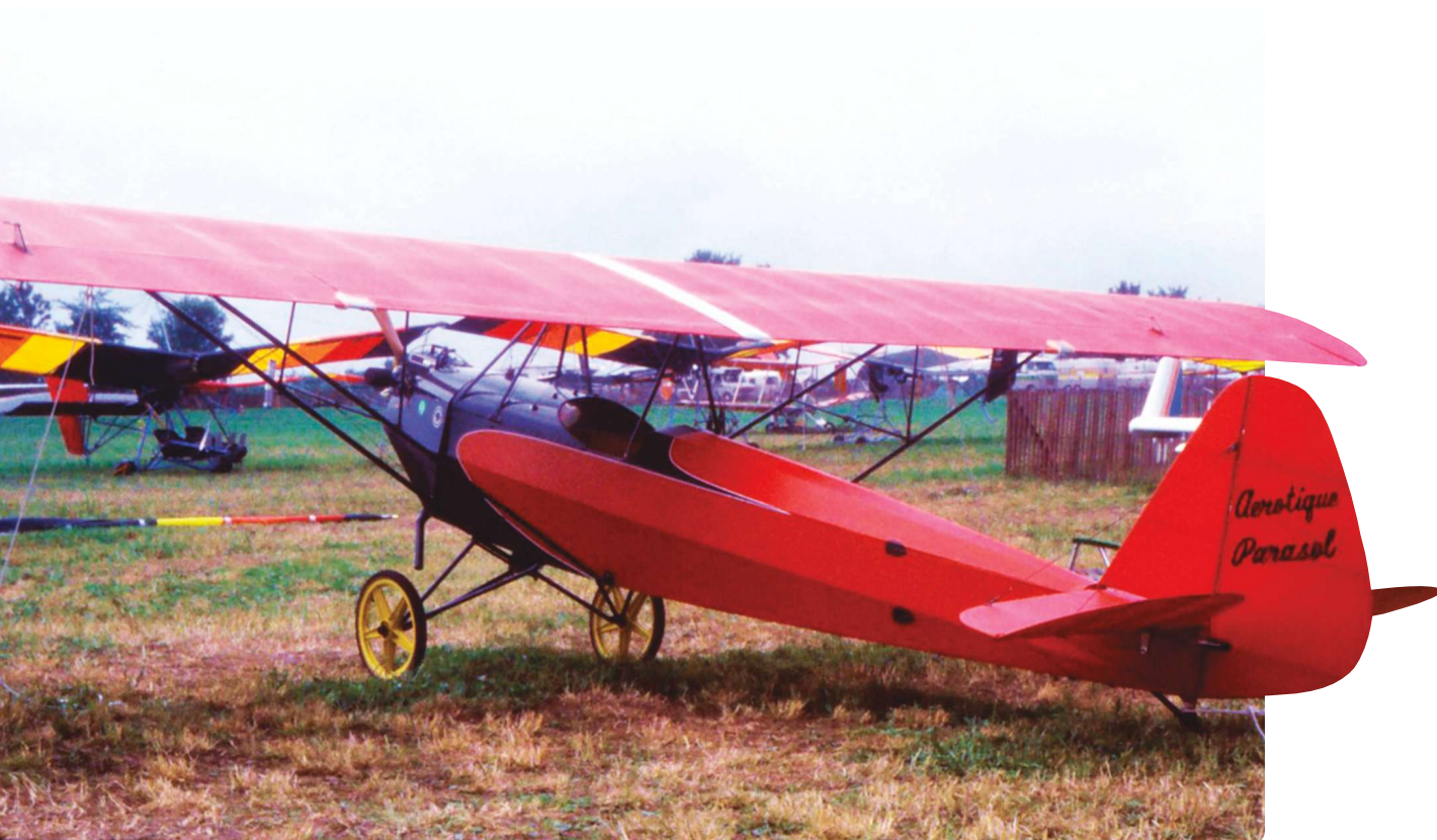
Aerotique Parasol by Stan Truman at Oshkosh '83 was designed as an ultralight version of the 1926 Heath Parasol.
