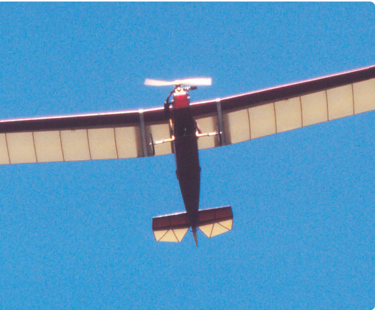
Cantilevered wing of the plans-built Sky Pup viewed from below.
