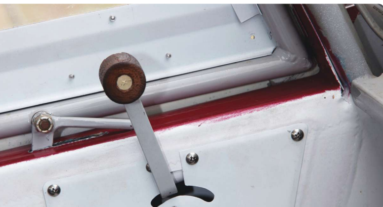
The elegantly simple throttle is now controlling a 100-plus hp engine that is a combination of Continental C-85/O-200 parts.
