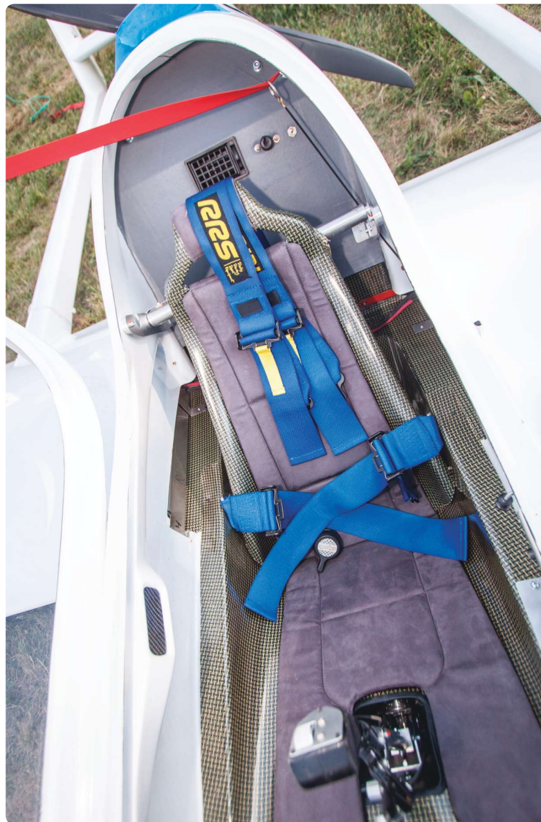
The ULS’ interior is constructed of carbon and aramid materials. The rudder pedals and seat back are adjustable to accommodate pilots of any height. A four-point seat/shoulder harness are standard equipment.
