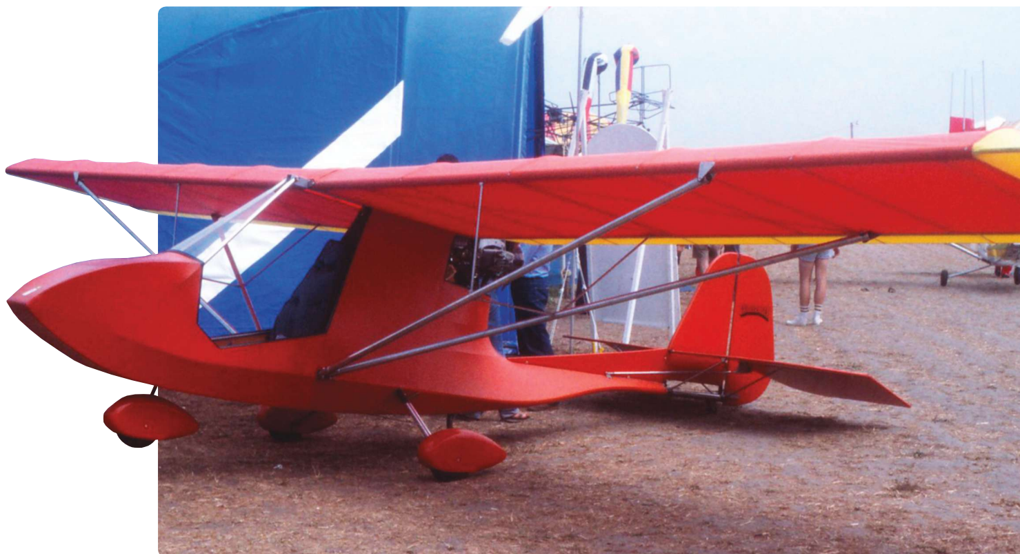
The original Challenger ultralight on display at Oshkosh '83 was powered by a 25-hp KFM engine.
