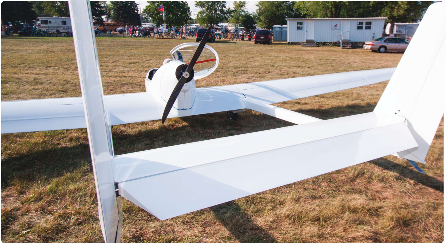
This view shows the standard fixed two-blade prop that comes on the ULS, as well as the twin rudders. Fishman discusses his ElectraFlyer ULS in this video.
