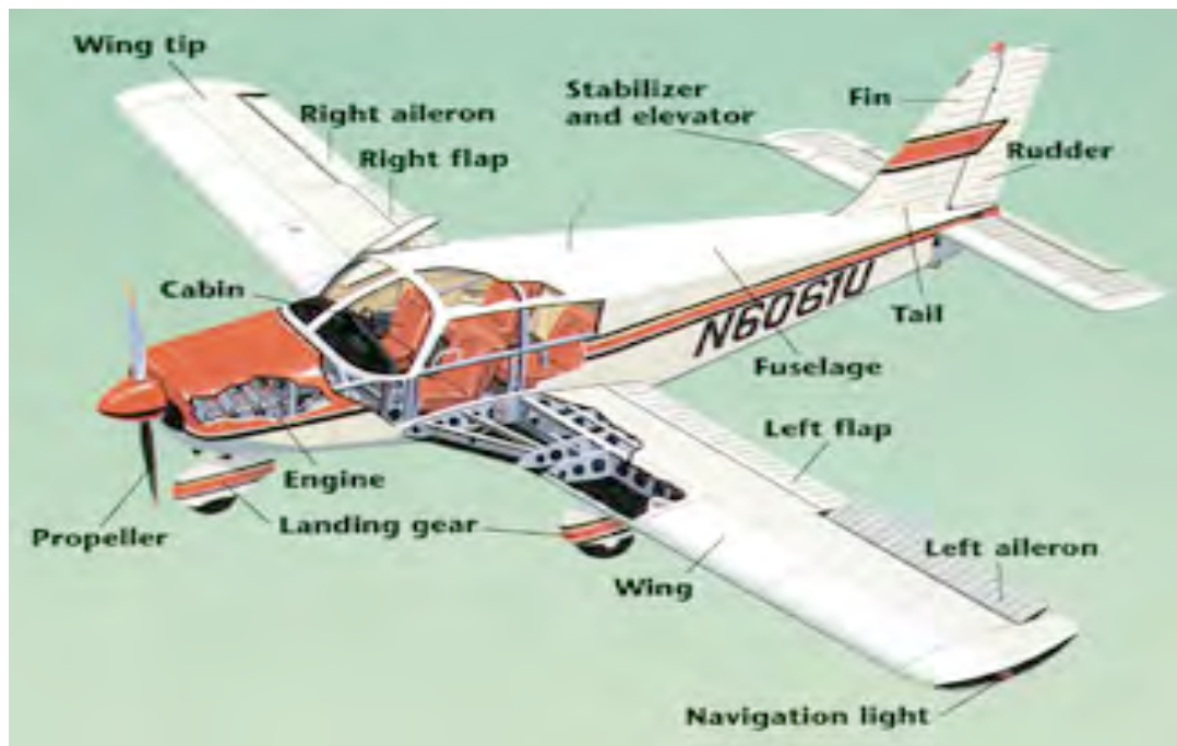
Image above: This drawing shows the parts of a light airplane called a Piper Cherokee.
