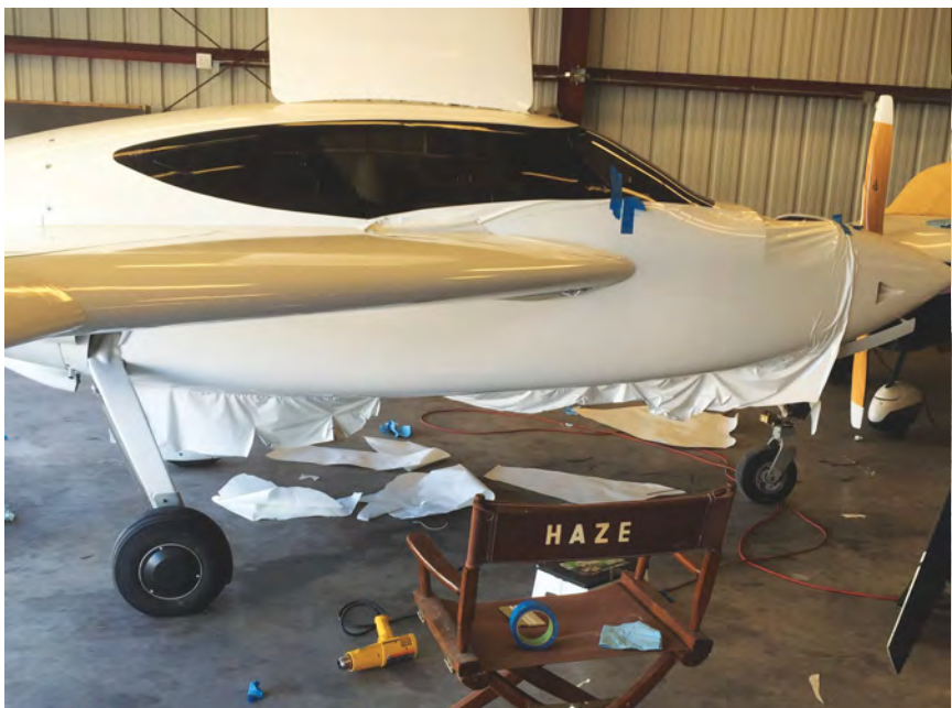
Above: The vinyl stretches to conform to the shape of whatever you're applying it to. Below: The Avery vinyl uses a pressure-sensitive adhesive allowing for repositioning over large areas.
