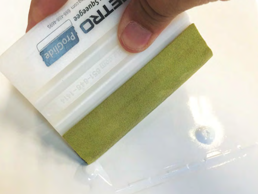
A felt-tipped squeegee was used to apply the vinyl to prevent scratches.
