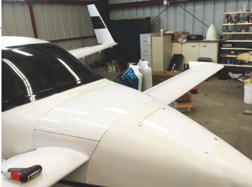
The access panel on the nose was the first section to be vinyl wrapped followed by the panel over the canard wing.
