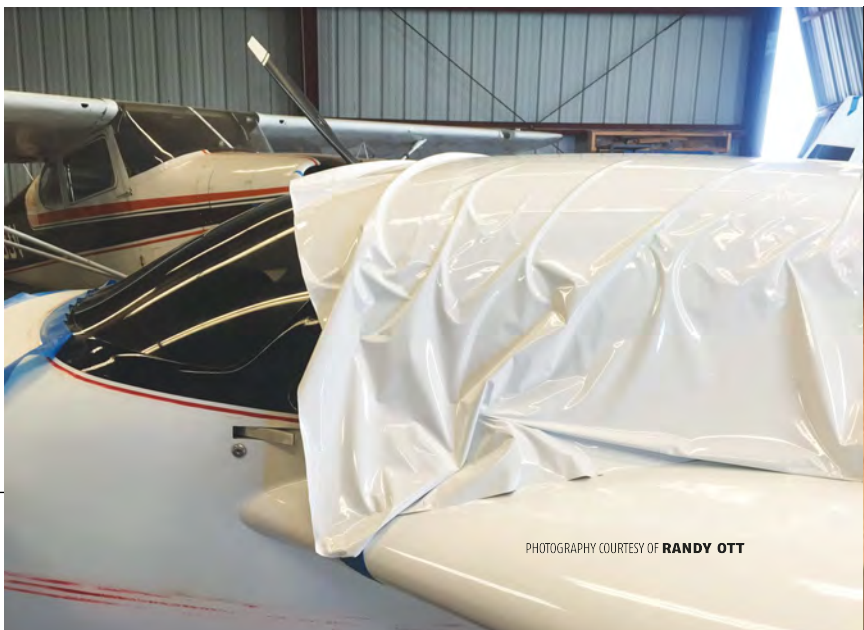
Above: The vinyl stretches to conform to the shape of whatever you're applying it to. Below: The Avery vinyl uses a pressure-sensitive adhesive allowing for repositioning over large areas.
