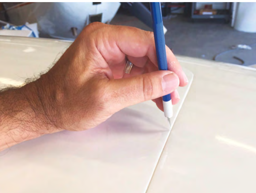
Above: I used an X-Acto knife to trim unneeded material before application. Below: A heat gun can be used to restore the shape of the vinyl if wrinkles appear.
