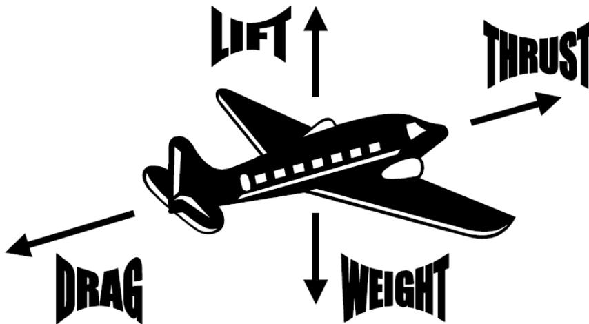
**Drag:** *The air resistance that tends to slow the forward movement of an airplane due to the collisions of the aircraft with air molecules.*
