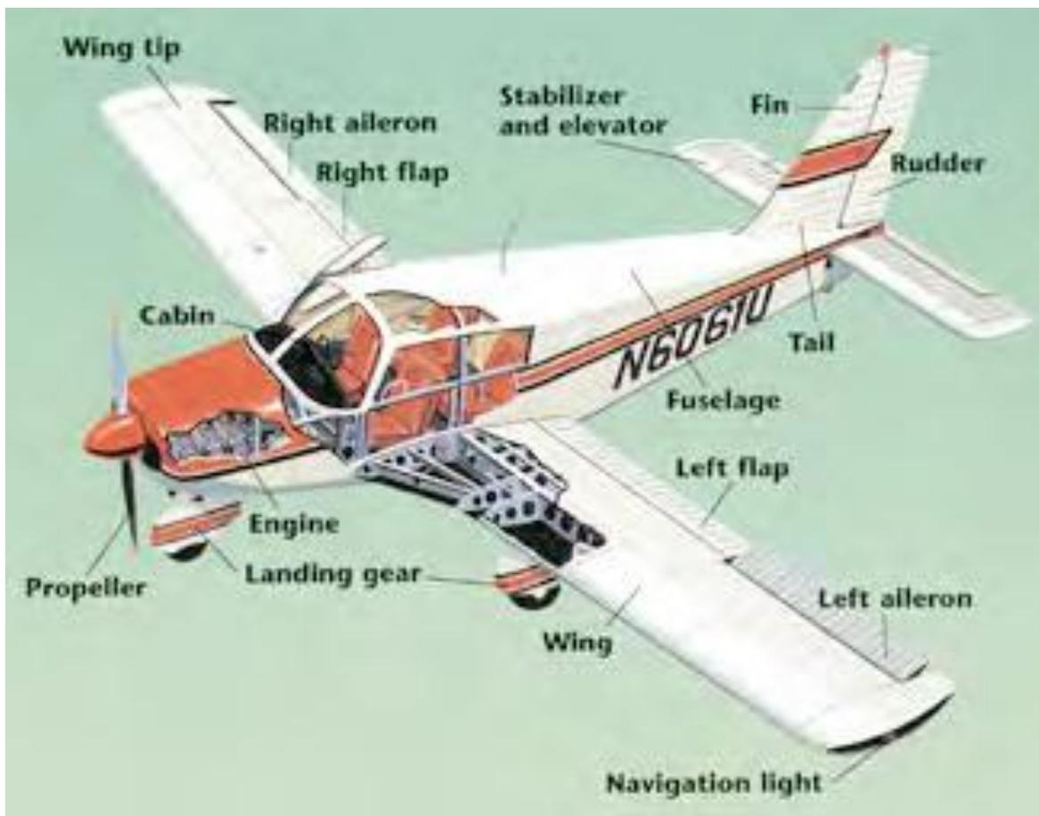
Image above: This drawing shows the parts of a light airplane called a Piper Cherokee.
