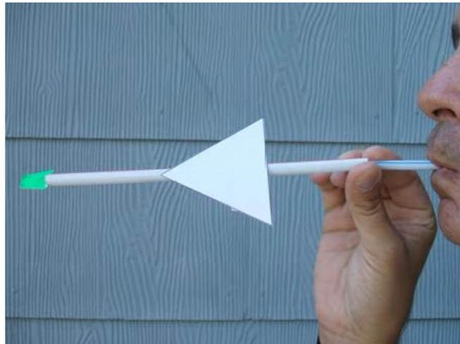
6. If the front of the jet rises, wrap some tape near the front of it until it flies level. If the front of the jet falls, wrap some tape around the straw just behind the wings.
