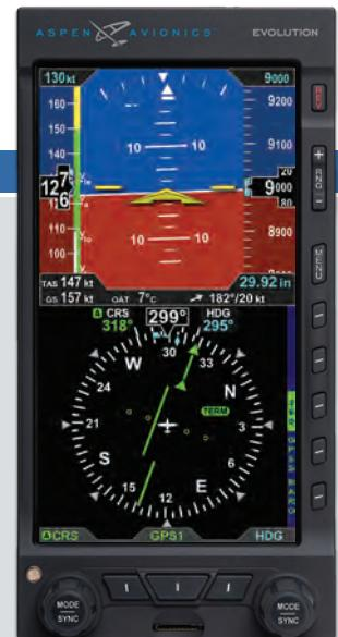
Evolution E5 Dual Electronic Flight Instrument
