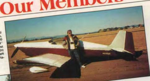
Left — This low profile Jodel F12 was a first project for Bill Sjöberg, 500 SW 329th St., Federal Way, WA 98023. Power is with a Lyco O-235-C1 with a 76x52 Sensenich prop. Cruise speed is 120 mph. The Jodel is constructed of birch ply and spruce and has a one piece wing. Bill has 45 hours on the Jodel and calls it Belle Etoile, French for Beautiful Star.
