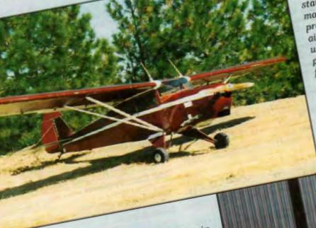
Right - "First flight of my RV-6A was in November 1992. Construction took 25 months. It is equipped with an O-320-D1A Lycoming engine. Gear leg fairings are glassed as part of the leg structure. The Hendrickson wood prop is a 'mostly cruise' propeller."
