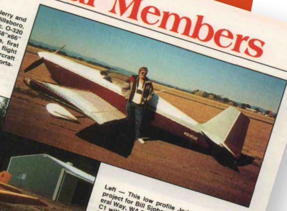
Left — This low profile Jodel F12 was a first project for Bill Sjoberg, 500 SW 329th St., Federal Way, WA 98023. Power is with a Lyc. O-235-C1 with a 76x52 Sensenich prop. Cruise speed is 120 mph. The Jodel is constructed of birch ply and spruce and has a one piece wing. Bill has 45 hours on the Jodel and calls it Belle Etolie. French for Beautiful Star.
