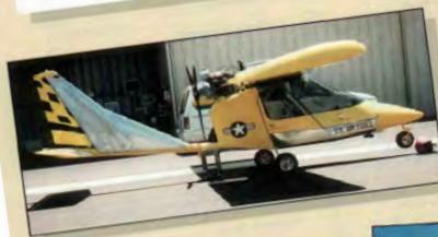
"I completed this RV-8 from Van's builder friendly pre-drilled kit in one year of determined part-time effort with some modifications. Engine and prop are from Van's — O-360-A1A and Hartzell constant-speed. Performance is to specs and is very enjoyable to fly. Special thanks to Jason Baranek, area builders, and Bob Baker of Bakersfield Municipal for a superb paint job."
