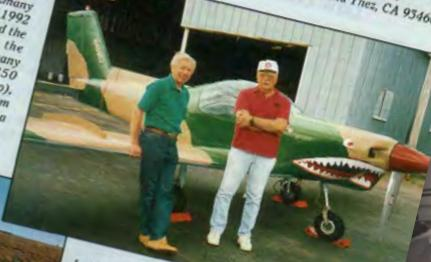
Left - "I built my wide body, folding wing Thorp T-18 over a period of 14 years. The plane, equipped with a 180 hp Lycoming engine and constant speed prop, has wet wings (17 gals each side) and electric elevator and aileron trim, electric flaps, and a landing light in each wing. It is also fully IFR including a horizon, attitude indicator, and a fuel gauge. The plane cruises at 180 mph and has a range of 1,000 miles."
