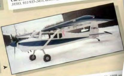
"My Titan Tornado entered service on May 31, 1999 and had a maximum speed of 120 mph and a cruising speed of 105 mph. Best rate of climb is 1,100 fpm at 65 mph. Full throttle is 120 mph. It burns 2.7 gph and will go 100 miles on 10 gallons of auto gas. The quality of the kit was outstanding, and factory support was quite good. Also have a BRS chute installed."
